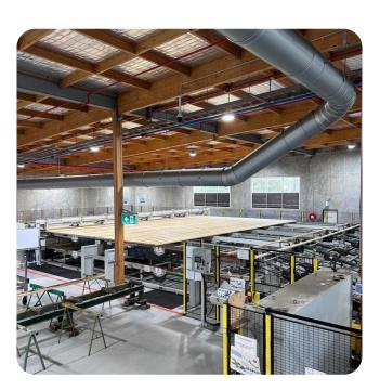
**Hyne Timber GLT** at Maryborough manufactures Australian timber GLT products in a fully automated facility. Undergoing a significant upgrade in 2020, the facility features GLT structural beams in the internal fit-out that is combined with the fully automated technology.
